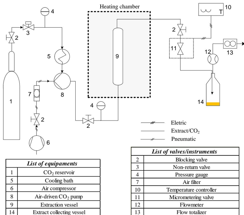
**Figure 3.** Flow diagram for the SFE-Spe-ed experimental apparatus (Adapted from Vasconcellos [8]).
