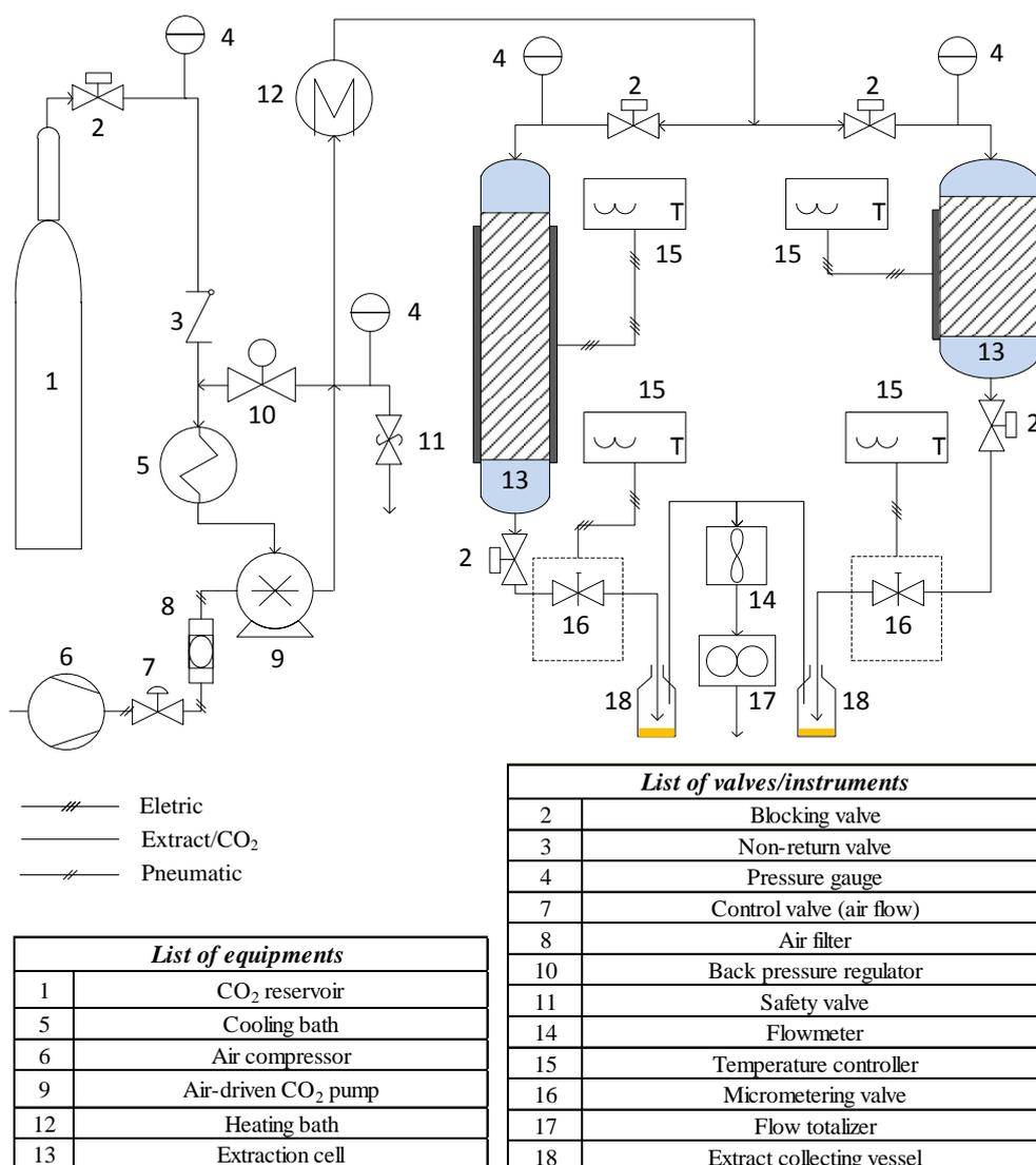
Figure 4. Flow diagram for the SFE-2x1L experimental apparatus.
