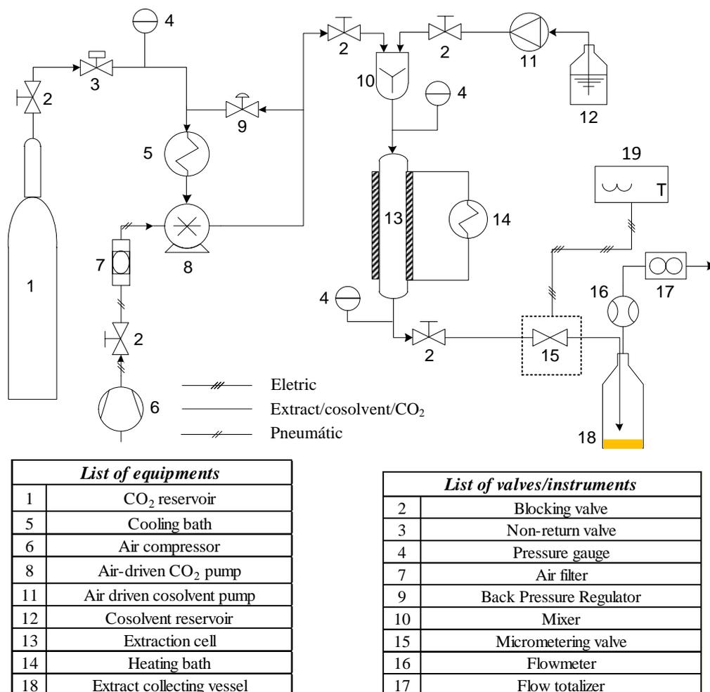
**Figure 2.** Flow diagram for the SFE-I experimental apparatus able to operate using cosolvent (Adapted from Veggi [4]).
