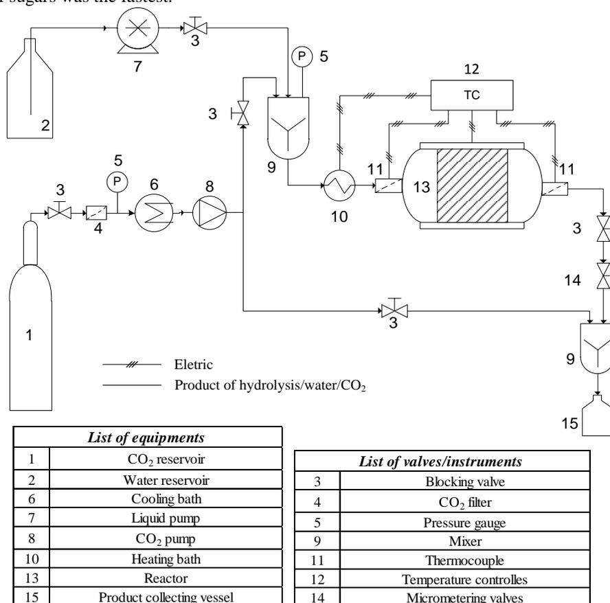
Figure 8. Flow diagram for the HYDRO experimental apparatus (Adapted from Prado *et al.* [20]).
