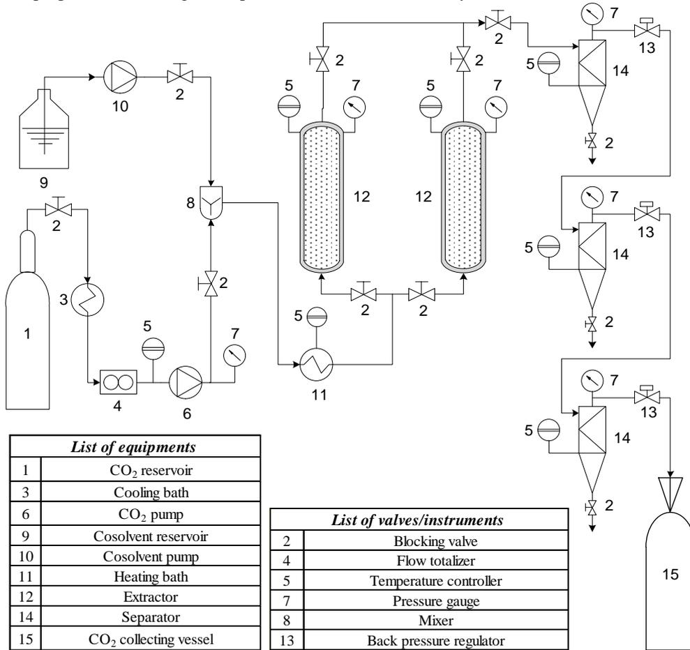
Figure 5. Flow diagram for the SFE-Pilot experimental apparatus able to operate using cosolvent (Adapted from Prado [14]).
