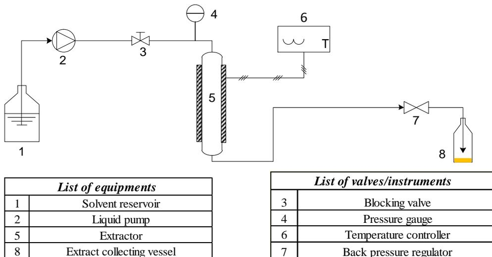
Figure 6. Flow diagram for the PLE-I experimental apparatus.
